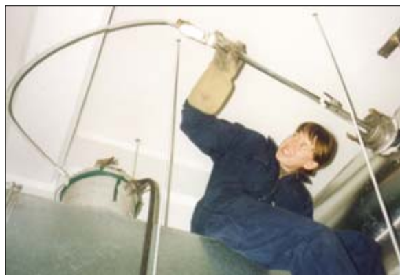
Deb at Purewa Crematorium inspecting the filter holder on the glass probe
