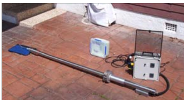
The new heated glass probe and controller
